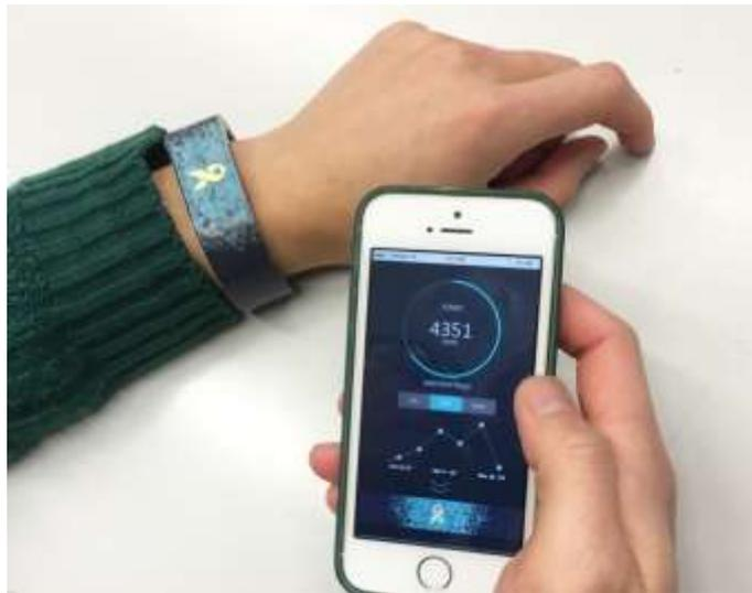
**Figure 5.** Model of the wrist-worn device and the mobile application of i-Ribbon (non-functional mock-up).
