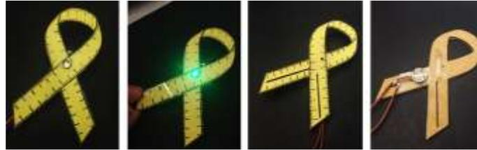
**Figure 3.** Two versions of the digital yellow ribbon, the first two pictures showing a concept based on visual output, the last two pictures showing the tactile output (vibration).
