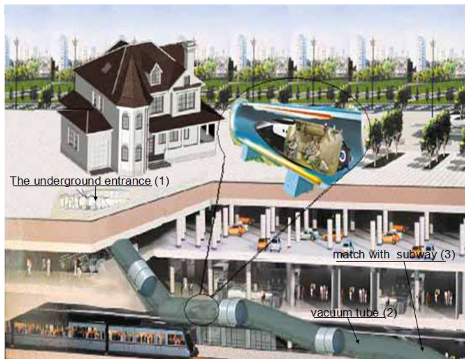
Figure 6. ST-I Transportation system - People enter the ‘ST-I’ in stage (1), stage (2) accelerates the passengers to match the subway speed, finally at stage t(3) passengers will transfer to the subway.
