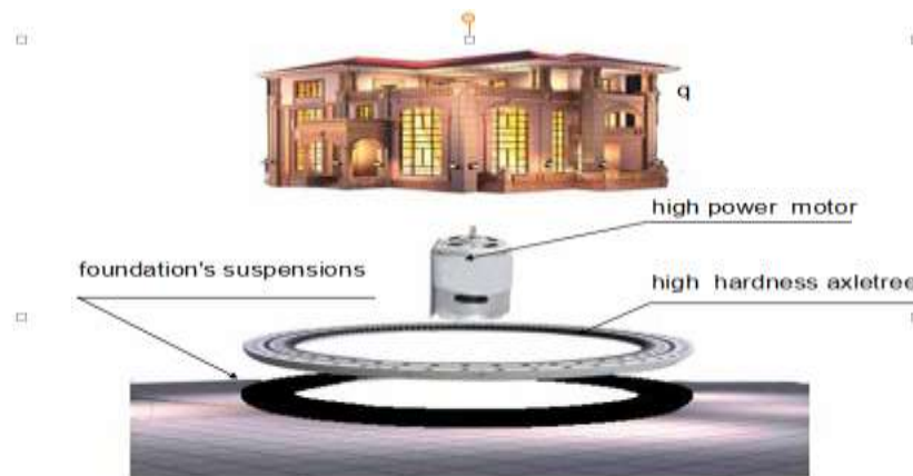
Figure 4. The foundation's suspensions and power system
